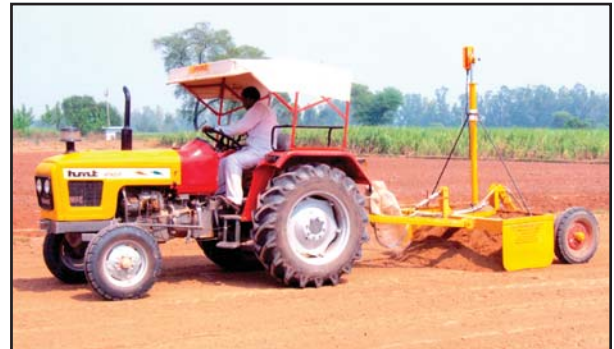
Fig. 1. Laser land levelling – Key to success of intercropping.
